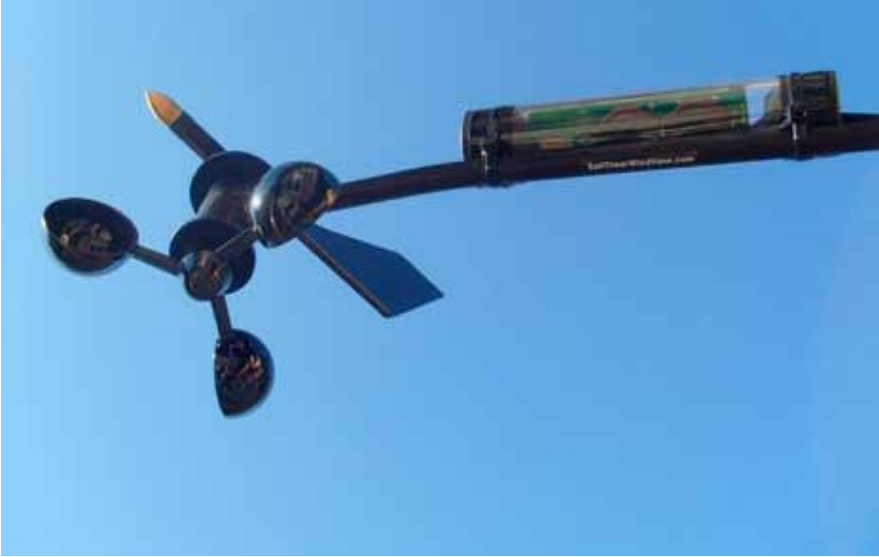
The SailTimer Wind Vane: wireless, solar-powered. Sends wind speed and direction through the air to an iPad, iPhone or The Sailing GPS. From www.SailTimerWindVane.com
