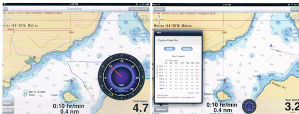
"Large wind speedometer in the SailTimer app (left). Custom polar plot learning (right) allows more accurate results for optimal tacks and Tacking Time to Destination."
